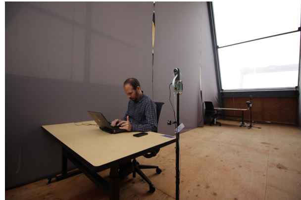
Figure 9 – A photo of a test subject in one bay of the mockup. The equipment stand at the corner of the desk holds the raspberry pi camera and horizontal illuminance sensor.
