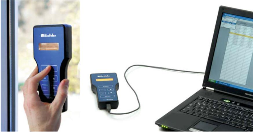
**Fig. 5.11** Example of thickness gauge for glass (courtesy of *Glass Buddy—Bohle*)
