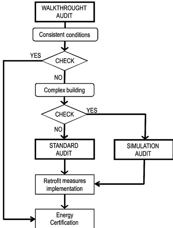
Through a walkthrough audit, we assess whether the overall energy consumption is high comparing with buildings of the same type. The same survey allows a first assessment of the ways in which plants are managed.
