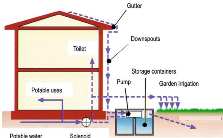
**Fig. 13.19** Schematic example of a rainwater harvesting system
