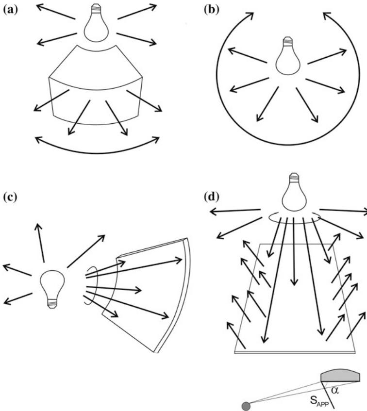
**Fig. 12.5** Fotometric quantities: (a) Luminous Intensity, (b) Luminous Flux, (c) Illuminance, (d) Luminance
