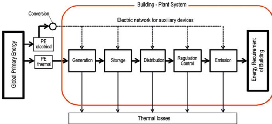
Fig. 8.4 Schematic diagram the subsystem sequence in a HVAC system
