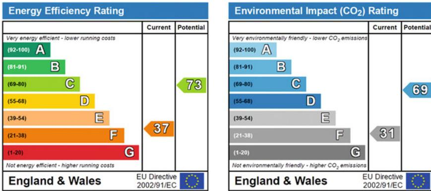
Fig. 2.2 Sample of energy performance certificate (Source SAP)
