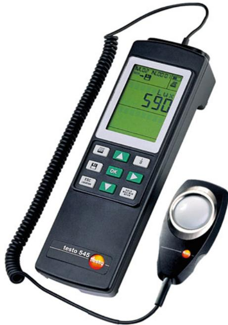
The instrument to be used for this purpose is the lux-meter that can measure the illuminance level expressed in *lux* (Fig. 5.9).
