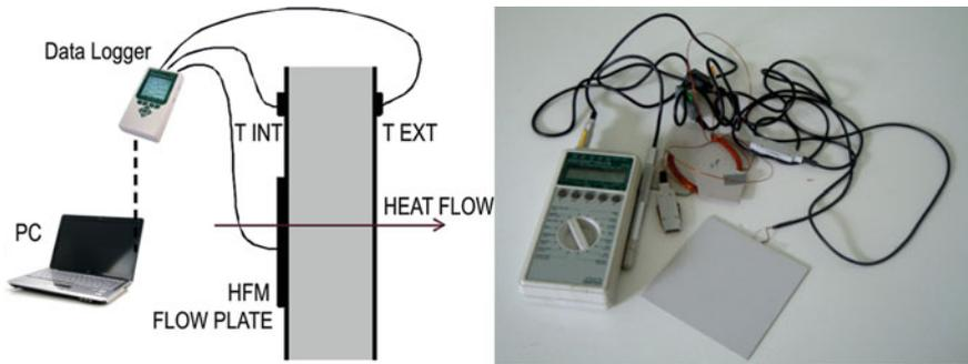
**Fig. 5.12** Installation scheme of a heat flow meter and example of a flow meter
