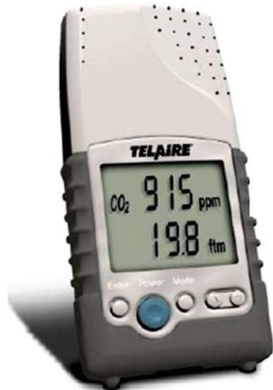
CO<sub>2</sub> concentrations of the outside air are normally between 250 and 350 parts per million (ppm). The presence of people within the confined spaces can be detected indirectly through the variation of this parameter.
