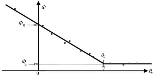
The values of the average power of the plant and the average outside temperature during the period are then plotted on a graph.
