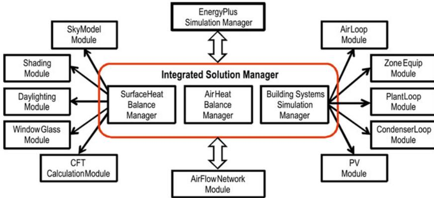
Fig. 7.3 The internal structure of EnergyPlus (Source Technical documentation EnergyPlus)
