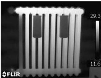
Infrared analysis can be efficiently used to verify the correct operation of a radiator. Looking at the thermal image, one notices a malfunctioning of the first element on the left which is still cold. This could be caused by over-pressurised inlet water.
