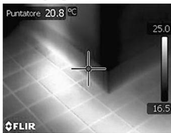
Through thermography, the professional operator can easily track water pipes, in order to act locally to a potential problem area and not by trial and error.
