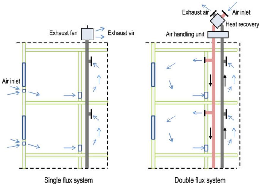
**Fig. 13.16** Typical schemes of mechanical ventilation systems
