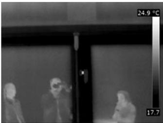
Not choosing the correct angle to minimise the reflections on the thermal image could lead to an erroneous temperature acquisition. The image on the left shows the reflection of IR radiation from three people on the window being analysed.
