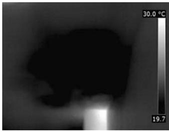
The thermal image on the left shows a water stain on a ceiling: humidity and/or water infiltrations are generally colder than the rest of the technological item under consideration, owing to the cooling effects of evaporation.
