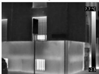
The image on the left is emblematic for understanding the way to recognise thermal coating: the lower part of the wall is clearly hotter than the upper part, owing to the absence of thermal insulation. Structural elements are also easily identifiable, while the coated part of the wall has very uniform temperature.
