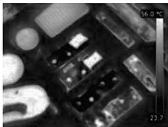
Different objects at the same temperature but with different emissivity coefficients are shown with a different temperature contour by the thermal image.
