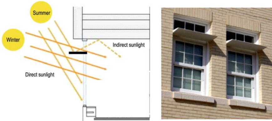
**Fig. 13.13** Example of an application of light shelves
