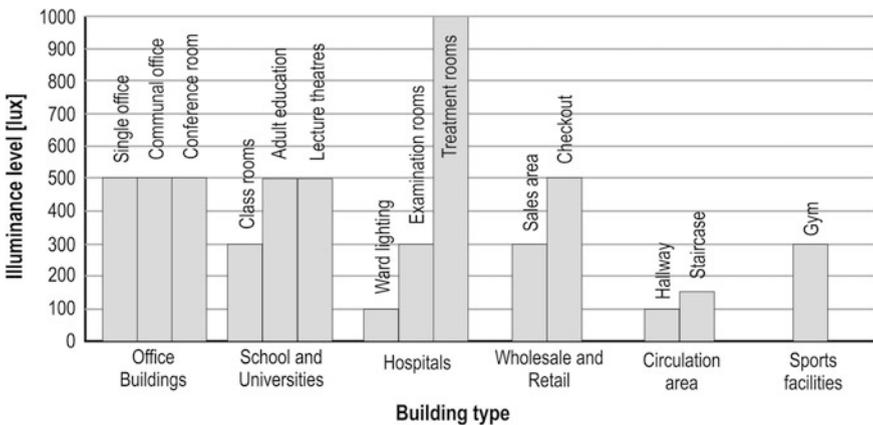
Fig. 12.6 Illuminance levels for different user applications [13]
