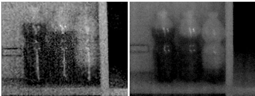
**Fig. 6.4** Same scene, different IR camera Thermal Resolution. The coarse-grained thermal image on the *left* was taken by an IR camera with a NETD value lower than the one on the *right*. Therefore, the instrument choice directly depends on the objective needs of the professional
