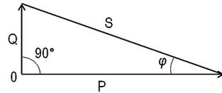
In a system with capacitive component, the phase shift is between 0 and  $-\pi/2$  (phase shift in advance). In both cases, the value of  $\cos\varphi$  power factor has a value lower than 1, with a minimum of (the theoretical value of) zero.
