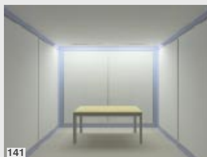
Recessed wallwashers with asymmetrical beam
