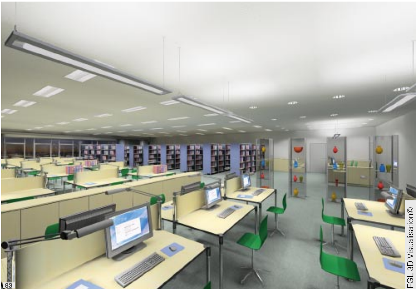
Nowadays, library searches are conducted on computers; card catalogues have all but disappeared. So lighting needs to be suitable for VDU use. VDU workplace luminaires designed for good glare suppression and direct/indirect lighting with electronic ballasts and high-grade louvers permit hours of searching without sore eyes.
