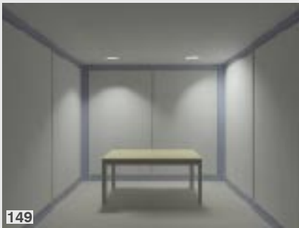
Downlights with symmetrical beam ( left ) or asymmetrical beam ( right )
