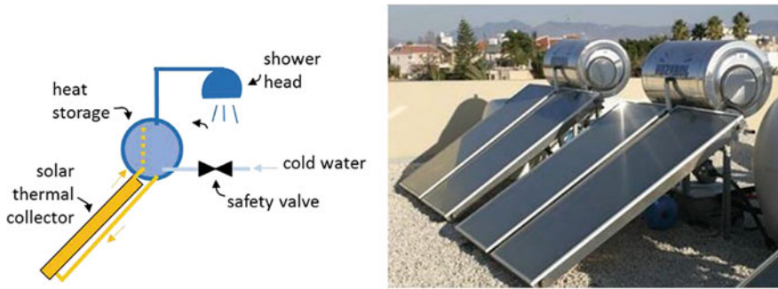
Fig. 10.11 Thermo-syphon DHW solar heating systems (SOLARGE 2004)
