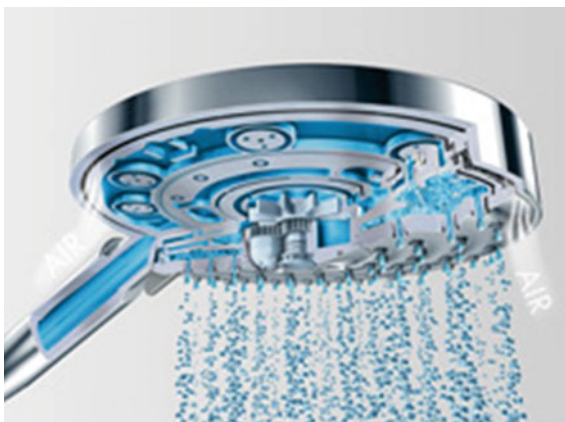
Fig. 10.10 Aerated shower head reduces water flow rate from 15 L per minute to 5–7.5 L per minute
