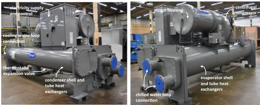
Fig. 9.14 Water-cooled vapour compressor refrigeration machine or chiller, full cooling capacity 123 MW c (350 ton), motor electrical power 250 kW e , rated COP 4.933 (Carrier, Evergreen 19 XR, Hermetic centrifugal water chiller)
