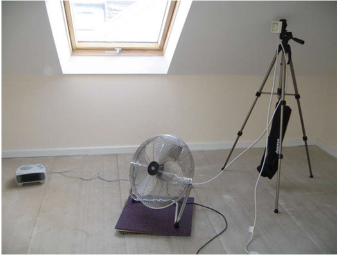
Fig. 4.16 During a co-heating method experiment, the building is maintained at a constant uniform and elevated temperature with electric heaters and fans installed in each thermal zone (space) in the building (Bauwens and Roels 2013)
