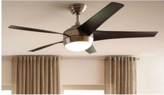
Fig. 1.7 During the cooling season, a ceiling fan blows air downwards and because of higher air velocity residents perceive lower indoor temperature (at 1 m/s a decrease of \sim 3 °C); if the tilt of the blades is changed during the heating season, the fan draws air up and reduces temperature stratification without the feeling of an unpleasant draught ( www.powerhousefan.com )
