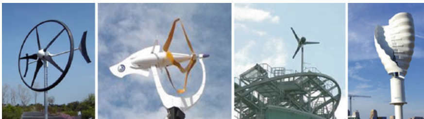
Fig. 7.27 Examples of small scale building-integrated wind turbines
