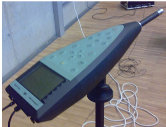
Fig. 1.16 Sound meter offer different methods for averaging of sound pressure level. Most common are 'F' (fast) or 'I' (impulsive) averaging
