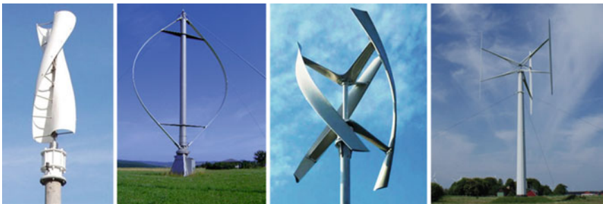
Fig. 7.25 Vertical axe wind turbines (VAWT) for near-by electricity production: Savonius rotor, Darrius rotor, helical rotor and H-type rotor
