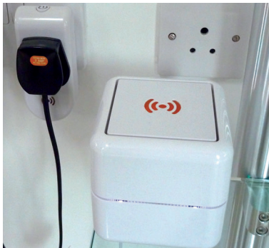
Figure 8.44 Whole house shutdown control can reduce energy consumption of appliances and devices (left).
