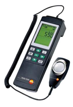
The instrument to be used for this purpose is the lux-meter that can measure the illuminance level expressed in lux (Fig. 5.9).
