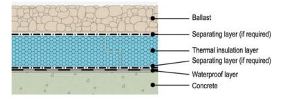
Fig. 13.4 Example of an inverted roof system (courtesy of Dow Corp.)
