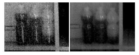
**Fig. 6.4** Same scene, different IR camera Thermal Resolution. The coarse-grained thermal image on the *left* was taken by an IR camera with a NETD value lower than the one on the *right*. Therefore, the instrument choice directly depends on the objective needs of the professional
