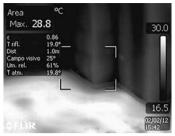
Through thermography the professional operator can verify, without contact, both the actual distribution of a floor radiant system and its correct operation.
