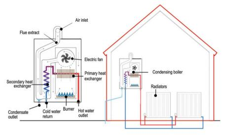
Fig. 13.14 Scheme of a condensing boiler and of a heating system (source: http://www.evoenergy.co.uk)
