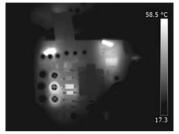
Infrared analysis permits clear recognition of which components of an electrical plants could potentially break down: looking at the thermal image on the left, of the three condenser in series, the central one has a higher temperature than the other two: clearly caused by a greater flow of electric current.
