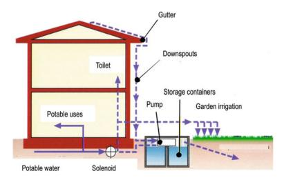
Fig. 13.19 Schematic example of a rainwater harvesting system
