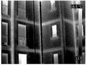
Thermal bridges are easily identifiable through infrared thermography: the different characteristics of materials give to each structural element a different temperature.
