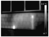
The thermal image on the left shows the uninsulated inlet and the outlet pipes of a radiator. They are clearly identifiable from the localised temperature rise on the exterior surface of the wall.
