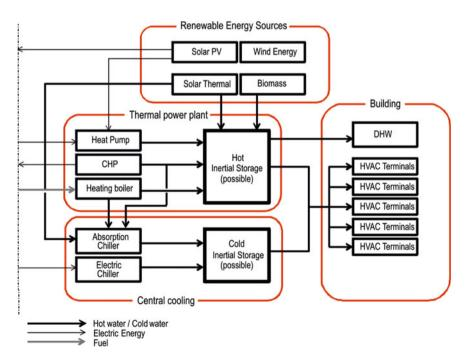
Fig. 8.3 Schematic diagram of a HVAC and DHW integrated system
