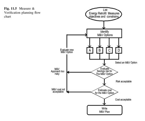
It is essential to first define the objectives and constraints of energy savings: based upon the type and complexity of the work: one of the four options for M&V is then chosen. The next step is the evaluation of savings and risk of the option.
