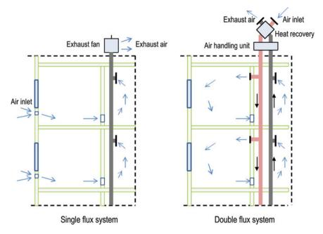
Fig. 13.16 Typical schemes of mechanical ventilation systems
