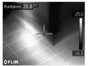
Through thermography, the professional operator can easily track water pipes, in order to act locally to a potential problem area and not by trial and error.
