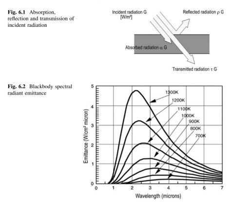
comparison in order to classify the characteristics of existing materials. In the real world there are no objects that are perfect absorbers, reflectors or transmitters. Therefore, the concept of a perfect blackbody is very important for infrared auditing, because it is the functional link between IR radiation and an object's temperature. This concept is reassumed by the Kirchhoff's Law, presented above [1].
