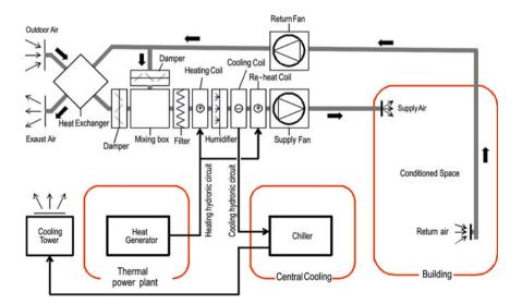
Fig. 8.5 Schematic diagram of a full air HVAC system
