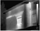
Through thermographic analysis it is possible to identify the external heat loss from radiators. In fact, it is visible because of a localised higher temperature on the exterior surface of the wall being considered (see the thermal image on the left, just under the window).
