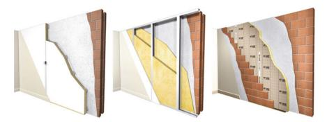
Fig. 13.9 Examples of internal insulation with counter-wall (courtesy of Isover Co.)
