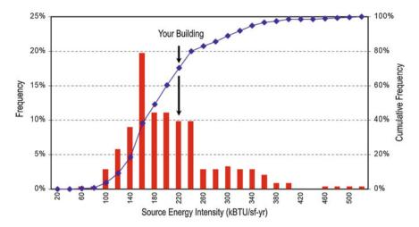
Fig. 4.3 Graphical representation of the results of a benchmark with Energy IQ Tool [4]
