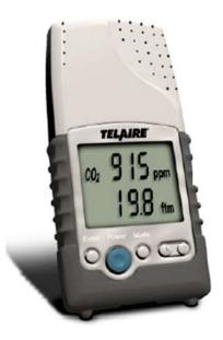
$CO_2$  concentrations of the outside air are normally between 250 and 350 parts per million (ppm). The presence of people within the confined spaces can be detected indirectly through the variation of this parameter.
