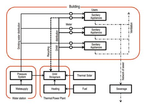
Fig. 8.6 Schematic diagram of a DHW system
