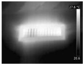
Infrared analysis could also be used to take the temperature of outgoing air from a vent.
