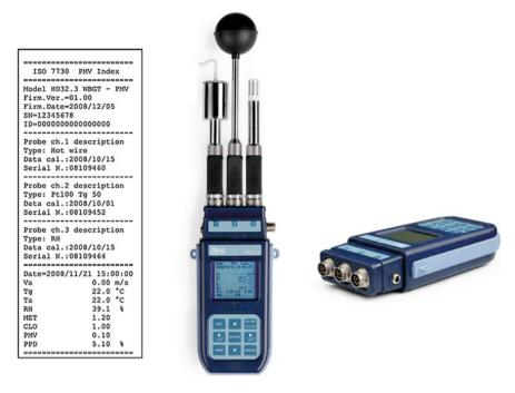
Fig. 5.7 Example of microclimate analyser (courtesy of Delta Ohm-www.deltaohm.com)
