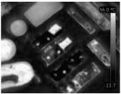
Different objects at the same temperature but with different emissivity coefficients are shown with a different temperature contour by the thermal image.
