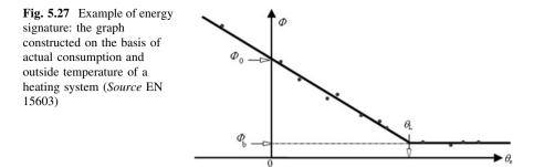
The values of the average power of the plant and the average outside temperature during the period are then plotted on a graph.
