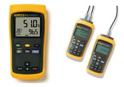
is sufficient to have a range between -10 and  $120 \,^{\circ}$ C), the measurement accuracy and the durability. The accuracy of the measurement mainly depends on the sensor that is employed. Almost all electronic thermometers are fitted with interchangeable sensors, which allows one to perform different measurements (e.g., air sensors, sensors for liquids, contact sensors etc.).
