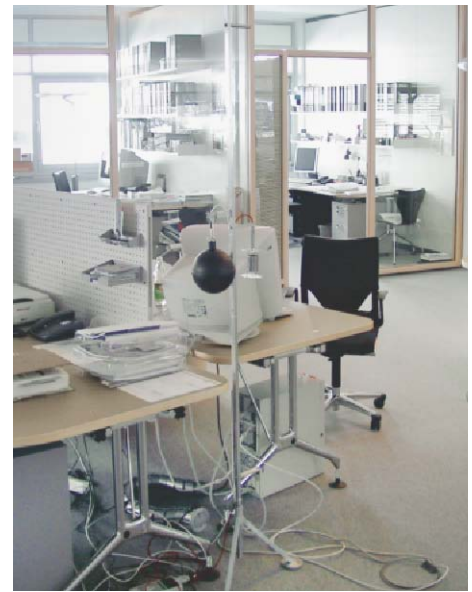
Fig. C3.5 Operative room temperature is measured with a bulb globe
