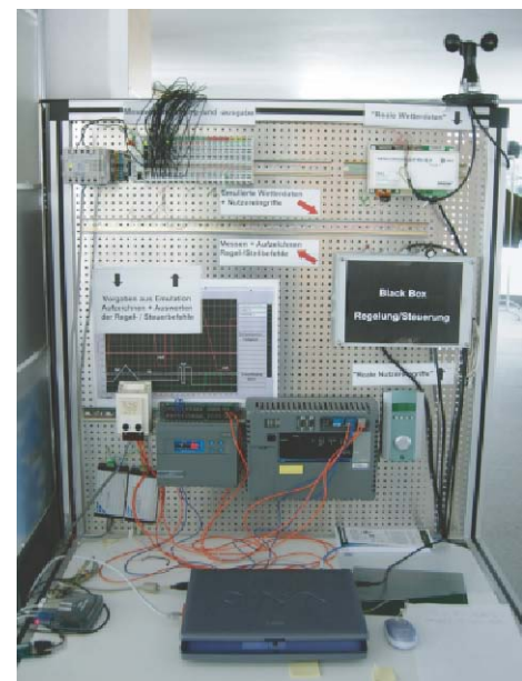
Fig. C3.13 Emulator set-up as a virtual test environment for realistic regulation and control components
