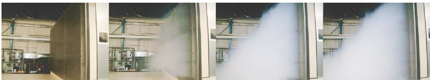
Fig. C.2.19 Airflow experiment at 1:1 scale at a fair hall at the Killesberg in Stuttgart
