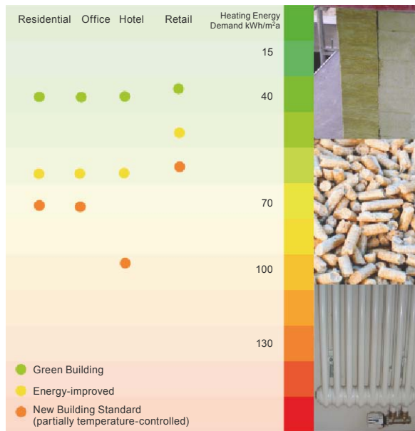
Fig. B2.7 Parameters for Heating Energy Demand in Central Europe, for different utilizations
