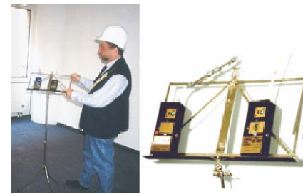
Fig. C3.7 Measuring air quality after building takeover
